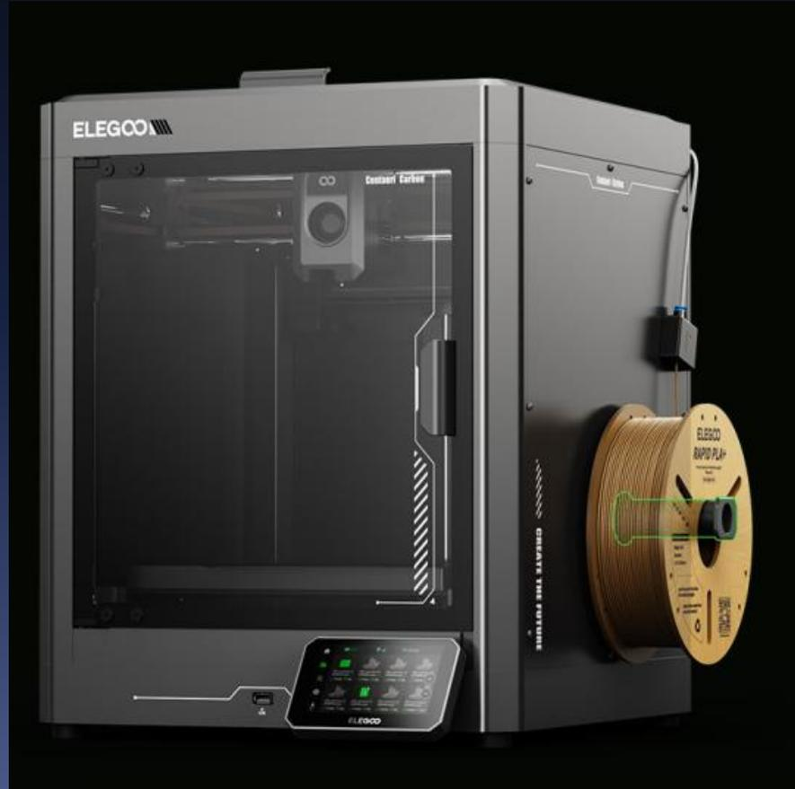
Most machines position the filament holder at the rear, making it inconvenient to replace the filament and monitor the remaining filament in real time.
